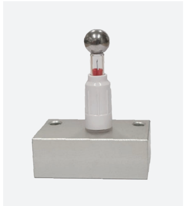
Placing a steel ball on the SPN and checking if the needle tip touches the surface of the steel ball.
