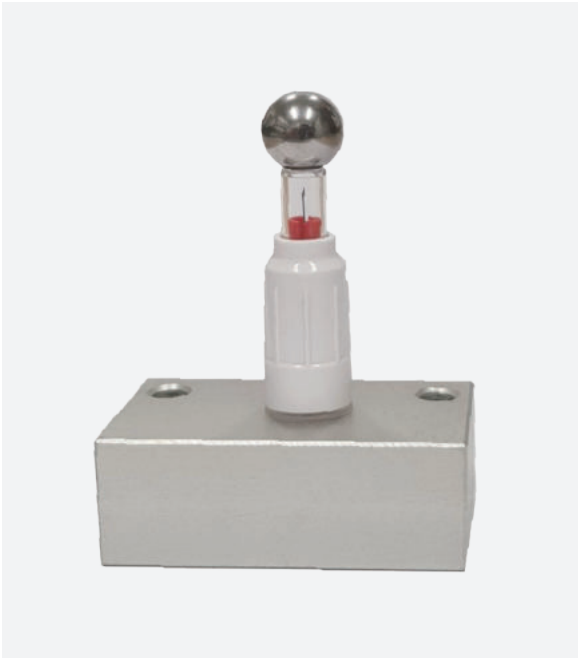
Placing a steel ball on the SPN and checking if the needle tip touches the surface of the steel ball.
